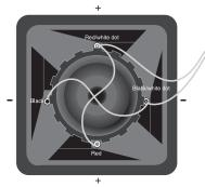
Dual 2 Ohm = 1 Ohm load Dual 4 Ohm = 2 Ohm load
